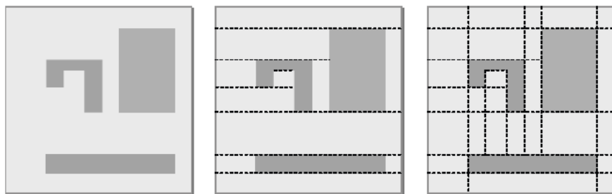
Fig. 5.17 Given a layout area with macro blocks (left), the horizontal (center) and vertical (right) macro-cell edges are extended to form the routing regions.
